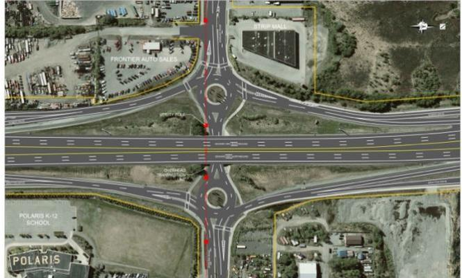
This project will take a fresh look at the Dowling Road/Seward Highway interchange by evaluating different interchange types and ultimately design a replacement interchange. The goal is to provide an interchange that serves both motorized and non-motorized travelers, is cost-effective, easy to maintain, and efficiently conveys both large and small vehicles. The reconstructed interchange will accommodate projected traffic volumes through 2040 and provide enhanced safety throughout the corridor.
